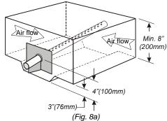
Horizontal duct with a minimum height of 8" (200mm)
