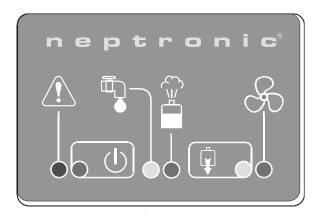
(Fig. 13) Front panel
