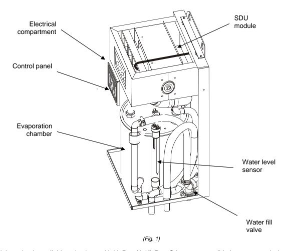
**SDU** module option is available only along with kit R or N. Kit D or S is non-compatible because no air duct is present. Please note that the APS supplied with standard Kit R will be substituted for an Air flow proving switch integrated into the **SDU** module.
