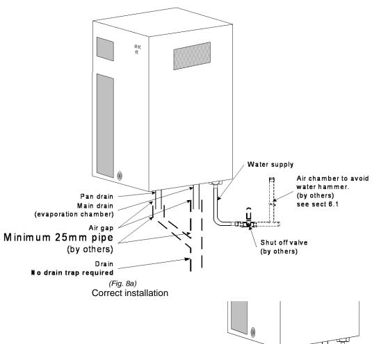
Main drain (evaporation chamber) must be straight.
