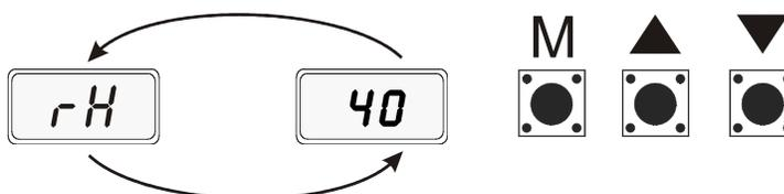
To proceed to the next level press **MENU** button.
