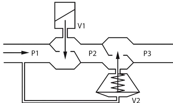
The diaphragm reacts to the system and regulates the pressure differential across the actuated control valve orifice to maintain its flow rate.
