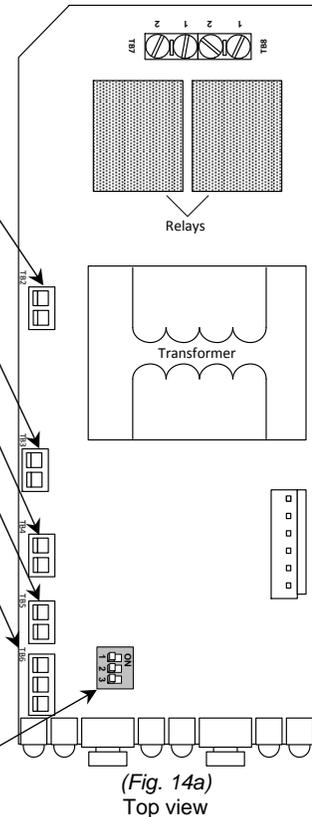
**10.2. P.C. Board for Modulating Humidifier**
