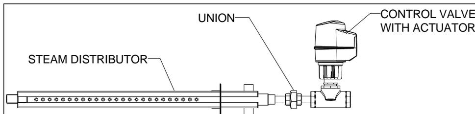
Illustration 10 - Control Valve Connection to Steam Distributor without Header
