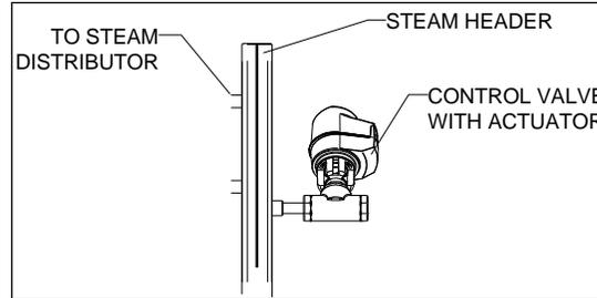
Illustration 11 - Control Valve Connection with Header
