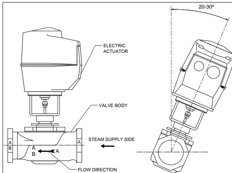
Illustration 9 - Control Valve Orientation and Angle
