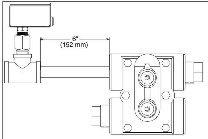
Illustration 20 - Steam Trap Installation: Distance from Temperature Sensor
