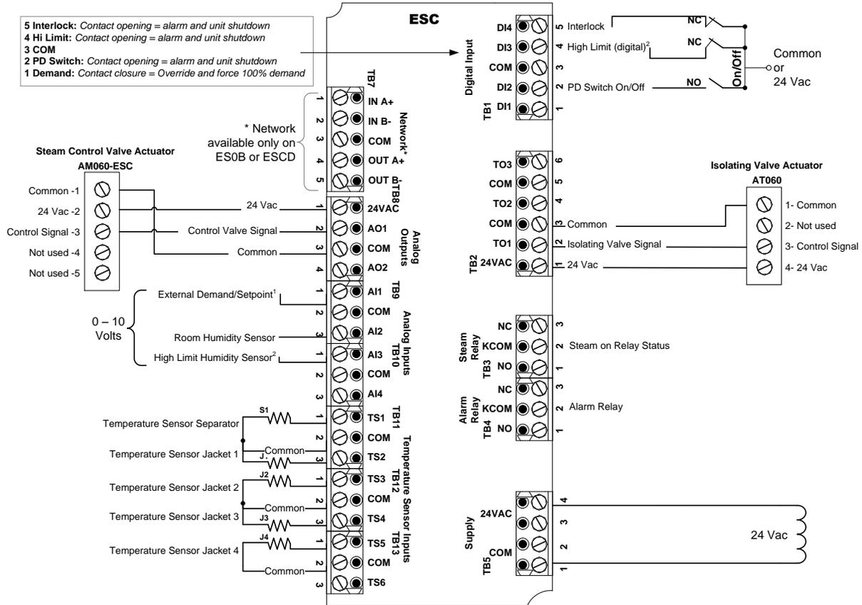
Temperature Sensor Jackets 1-2-3-4 sensor are optional, depending on system configuration.
