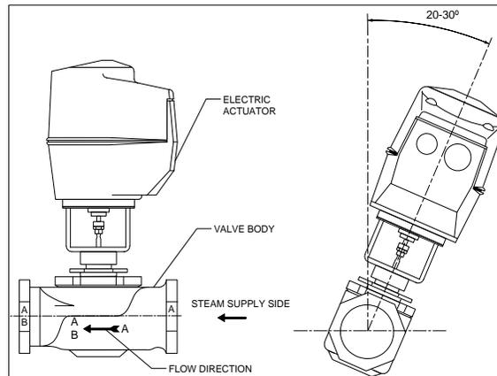
Illustration 22 - Isolating Valve Orientation and Angle
