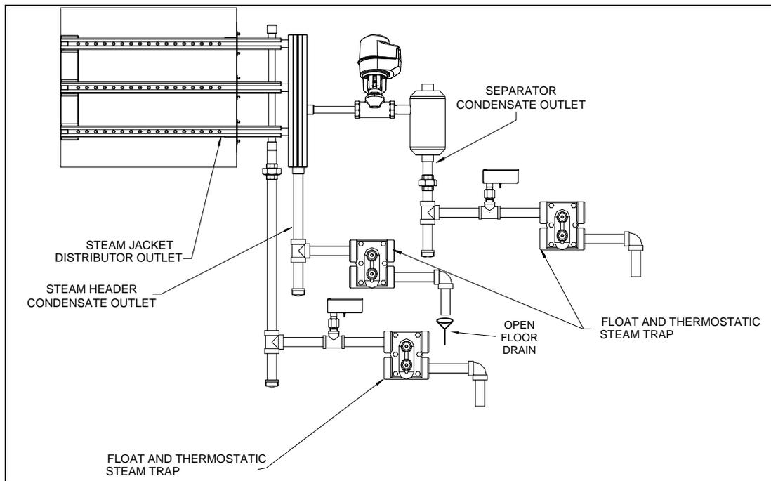
Illustration 21 - Steam Trap Installation (Mini Rack and Multi-Tube)
