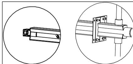
Illustration 6 - End Mounting Bracket and Escutcheon Plate
