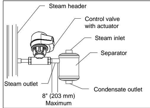
Illustration 16 - Separator Connection to Control Valve
