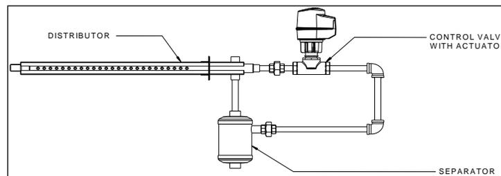
Illustration 14 - Single Steam Distributor Separator Correct Installation
