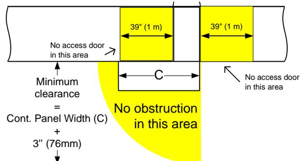
Provide a minimum clearance equal to  $C + 3''$  (76mm).
