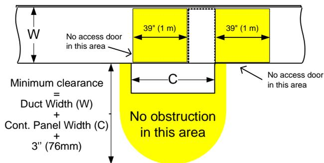
Provide a minimum clearance equal to  $W + C + 3''$  (76mm).
