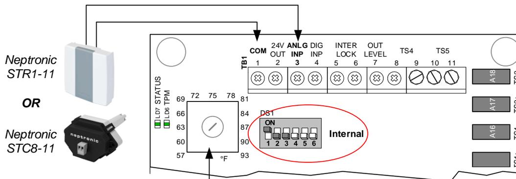
On-board setpoint: allows use of cost-effective sensor and setpoint is not accessible to the user. Requires HECF000P, HECF002P, or HECF005P
