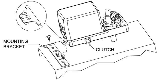
1. Manually close the damper blades and position the actuator to 0° or 90°.
