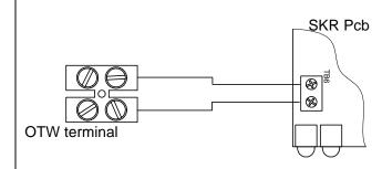
Connect **OTW** to terminal TB6 of the SKR Printed circuit board.
