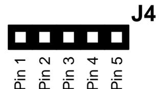
*When not used for programming, jumper is placed between pin 4 & 5*
