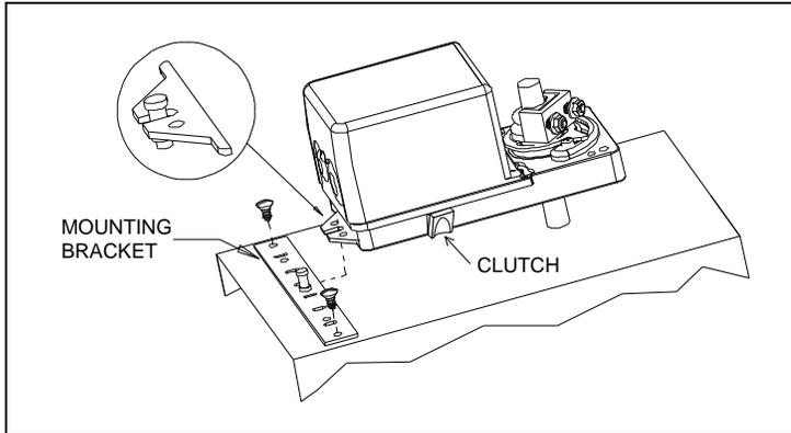
1. Manually close the damper blades and positioned the actuator at 0° or 90°.
