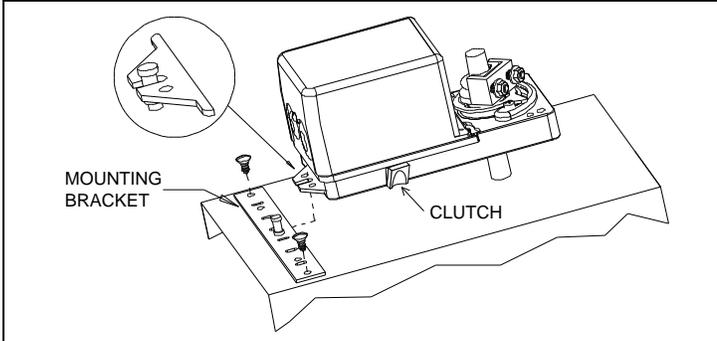
1. Manually close the damper blades and positioned the actuator at 0° or 90°.
