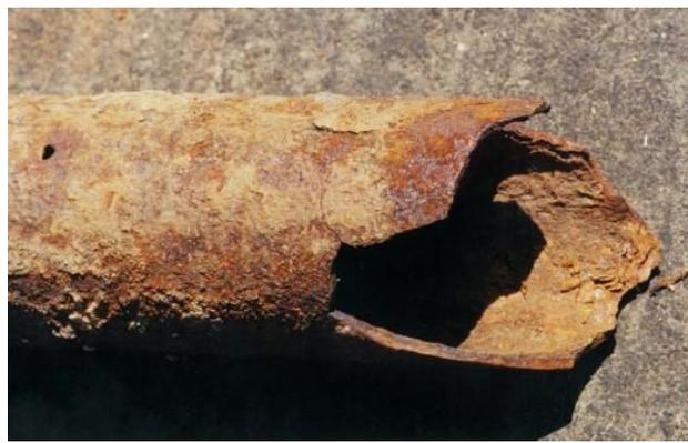
The acidic level of the condensate is measured in pH on a scale from 0 to 14. Most condensate will have a pH between 2.9 and 4 (according to the actual chemical makeup of the fuel that is being burned) with 7 being neutral. This scale is not linear; each step below 7 is 10 times more acidic than the next higher number. Treated condensate should be as close to neutral as possible with 5 being the minimum.
