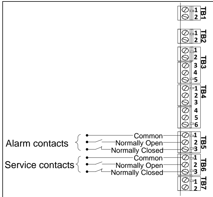
Illustration 40 - Alarm and Service Contact Wiring
