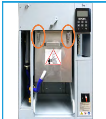
Disengage the 2 clamps
