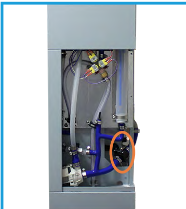
Disconnect the water inlet
