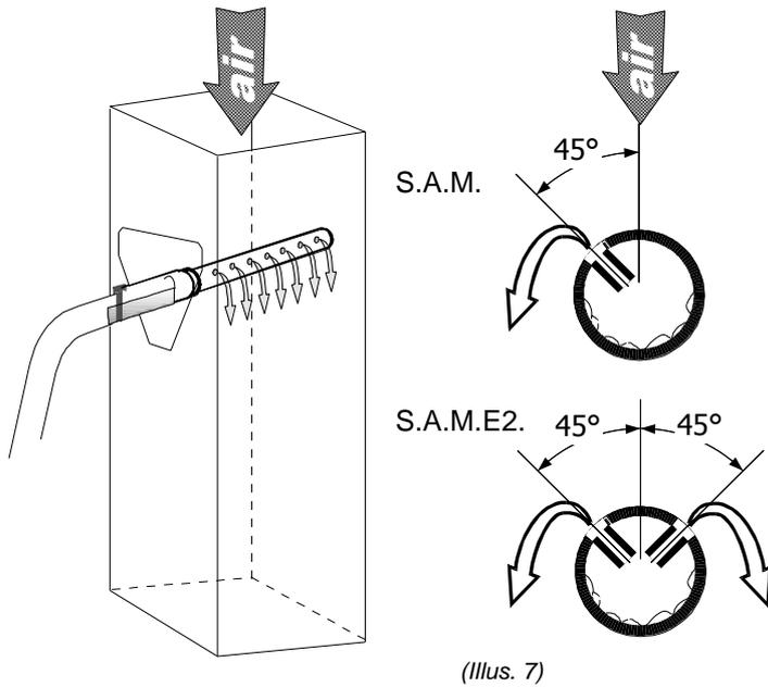
SAM or SAME2 for vertical ducts are used where the absorption distances are normal and the client requires an economical as well as an efficient solution.
