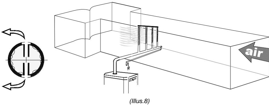
The Multi-Steam system is to be installed in critical locations in air handling systems, particularly where absorption distances are very short, less than 900mm, or low air duct temperatures are in effect.
