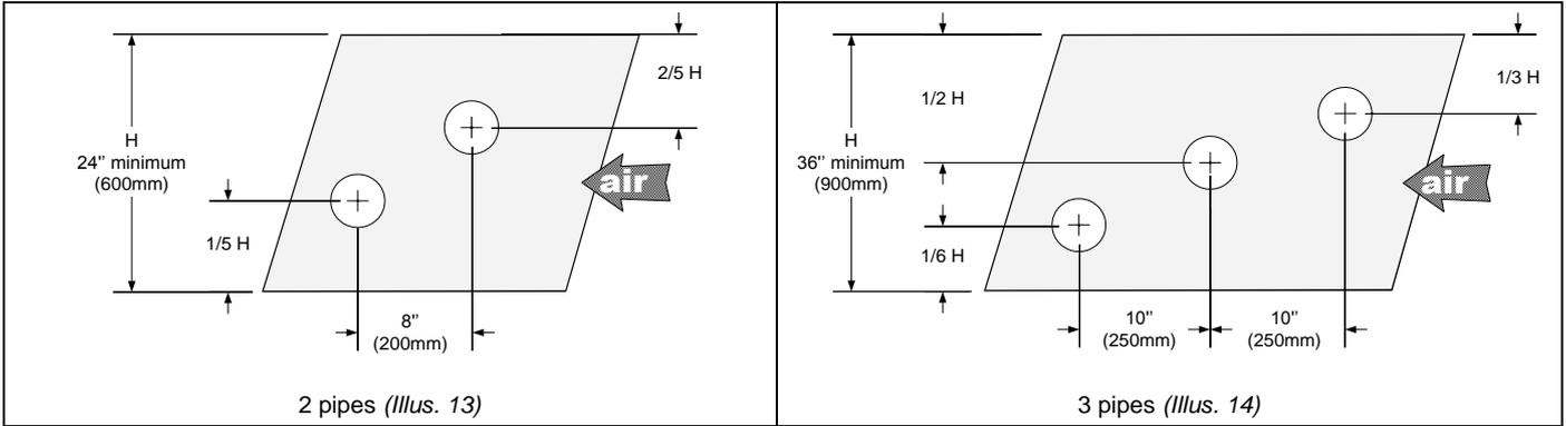
Note: 51 mm steam pipe must be supported on the end by appropriate duct hanger or strap (supplied by others).
