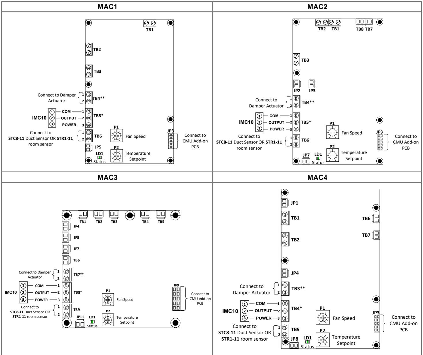
\* If the IMC10 Room Control Switch is not used, place a jumper or a dry contact for interlock between pins 1 & 2.
