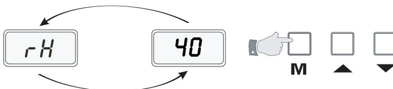
To proceed to the next level press **MENU** button. Otherwise, the humidistat will return to the control mode in 10 seconds.
