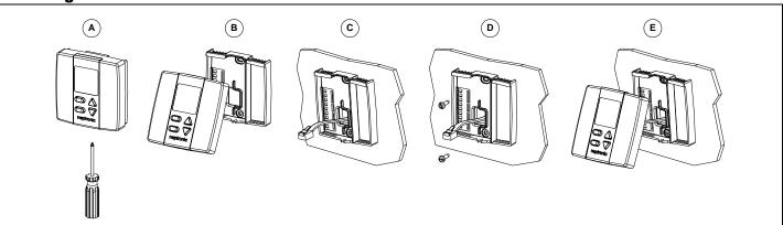
CAUTION: Risk of malfunction. Disconnect power prior to separating thermostat cover from its base.
