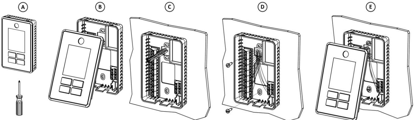
**i** Do not use the supplied screws to mount the unit to an electric box or an equivalent device. The supplied screws are only suitable for mounting the unit to the wall. Ensure to use the appropriate screws for any other application. Tighten by hand only and ensure not to overtighten the screws.
