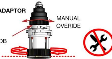
No foam insulation above the dotted line and around the adaptor
