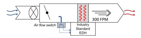
Open coil, modulating, max 50A
