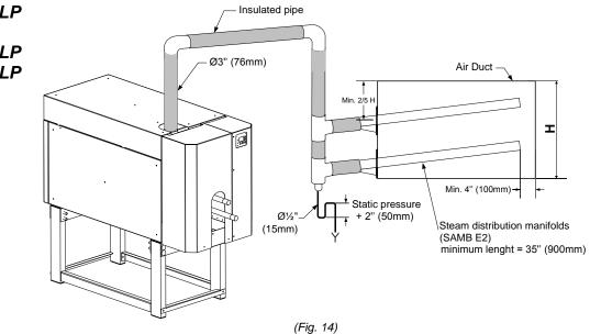
Single Ø3" (76mm) feed pipe must be connected to two (2) S.A.M.E2 Steam manifolds with a suitable reduction at the lowest point to allow a  $Ø\frac{1}{2}$ " (15mm) condensate drain from the main steam supply.
