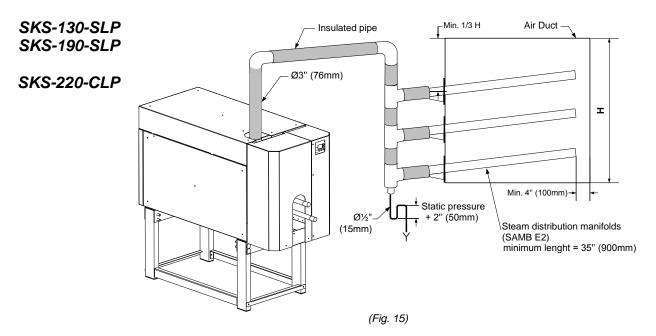
Single Ø3" (76mm) feed pipe must be connected to 3 S.A.M.E2 Steam manifolds with a suitable reduction at the lowest point to allow a  $\emptyset^{1/2}$ " (15mm) condensate drain from the main steam supply.
