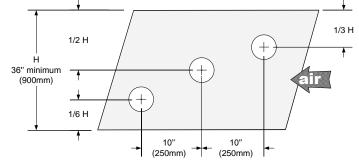
Horizontal duct – 3 manifolds (Fig. 9)
