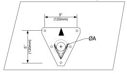
detail of manifold mounting bracket (Fig. 10)
