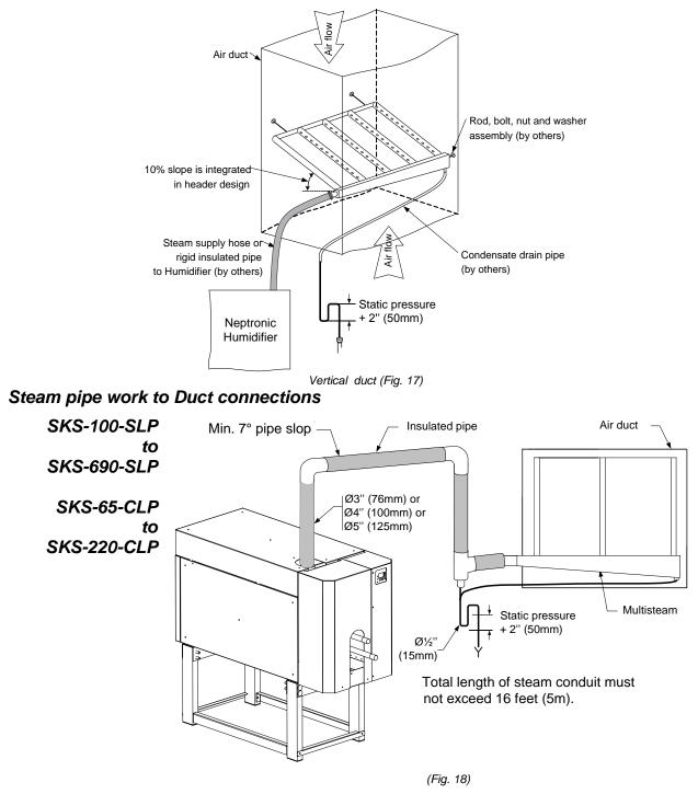
A single Ø3" [76mm] or Ø4" [100mm] or Ø5" [125mm] feed pipe must be connected to a single Multi-Steam with a suitable reduction at the lowest point to allow a Ø1/2" [15mm] condensate drain from the main steam supply.
