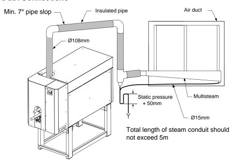
A single Ø76mm or Ø100mm or Ø125mm feed pipe must be connected to a single Multi-Steam with a suitable reduction at the lowest point to allow a Ø15mm condensate drain from the main steam supply.
