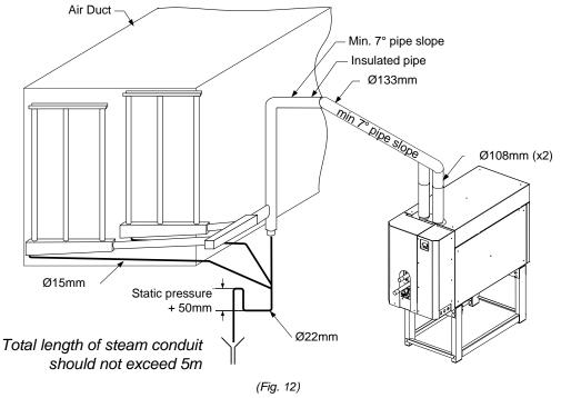
Two Ø100mm or Ø125mm steam outlets must be connected to two Multi-Steam with a suitable reduction at the lowest point to allow a Ø15mm condensate drain from the main steam supply.
