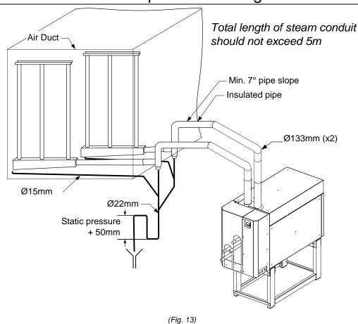
Two Ø125mm steam outlets to feed pipe must be connected to two Multi-Steam with a suitable reduction at the lowest point to allow a Ø15mm condensate drain from the main steam supply.
