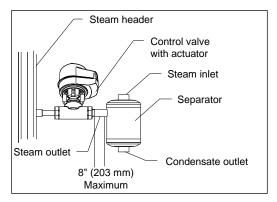
Illustration 16 - Separator Connection to Control Valve
