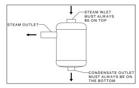
Illustration 12 - Separator Proper Installation
