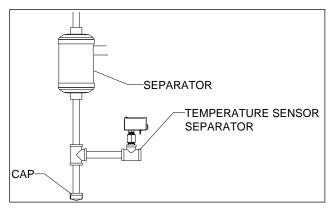
Illustration 17 - Temperature Sensor Separator Installation
