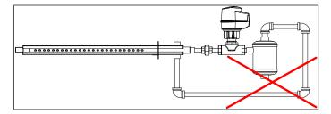
Illustration 15 - Single Steam Distributor Separator Incorrect Installation
