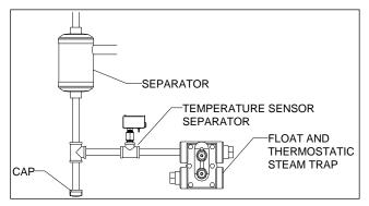
Illustration 19 - Separator Steam Trap Installation
