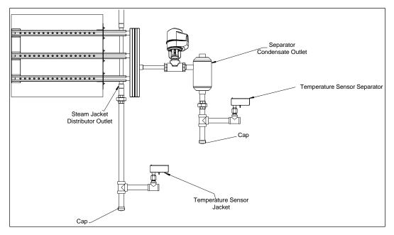
Illustration 18 - Temperature Sensor Jacket Installation
