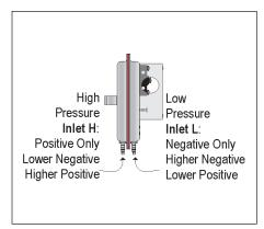
**Figure 2:** The sample line connections for typical applications.
