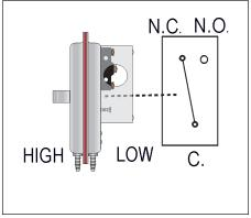
**Figure 3:** Before pressure is applied to the diaphragm, the switch contacts are in the normally closed (NC) position.
