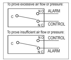
**Figure 4:** Before pressure is applied to the diaphragm, the switch contacts are in the normally closed (NC) position.
